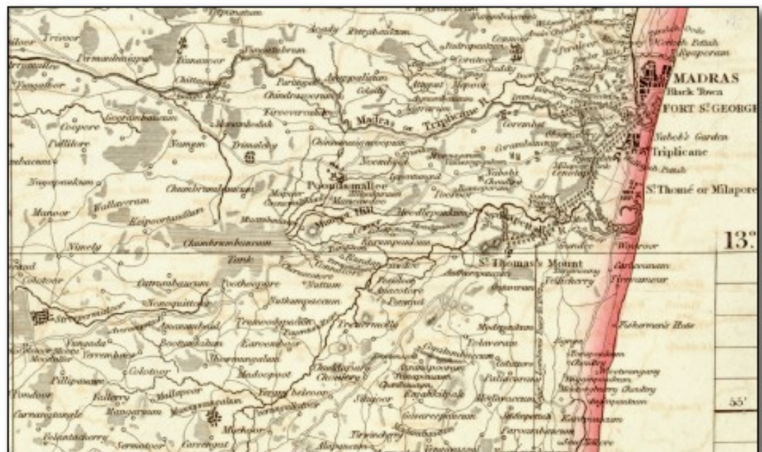
Figure 12. Arrowsmith atlas Madras sheet showing Lambton’s original 7 mile baseline, the northern end of which is at Guindy east of St. Thomas’s Mount, in the middle of the Chennai Race Course.
